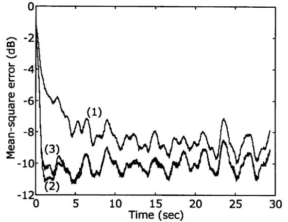
**FIGURE 4.** Learning curves for real signals: (1) FxLMS, (2) FxGAL and (3) combined lattice-transversal FxGAL.
