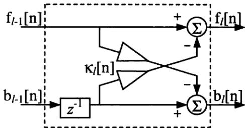
**FIGURE 1.** Detailed structure of  $l$ -th stage of an Adaptive Lattice Predictor.
