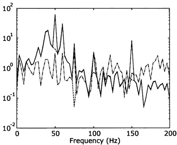
**FIGURE 5.** Error spectrums: ANC off (solid line), FxLMS with nonacoustic reference (dashed line), FxGAL with acoustic reference (dash-dot line).
