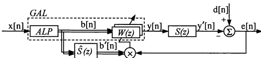
**FIGURE 2.** Filtered-x Gradient Adaptive Lattice (FxGAL) algorithm block diagram.
